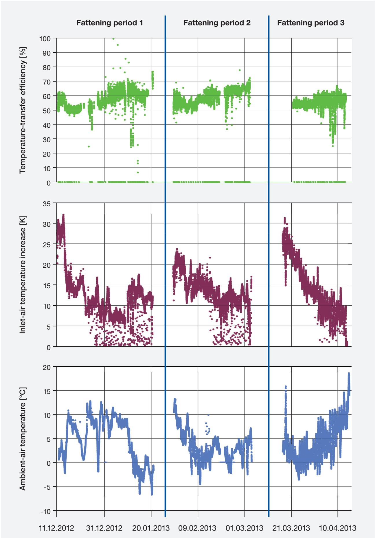
Figure 5: Temperature-transfer efficiency, inlet-air temperature increase and ambient-air temperature over time
