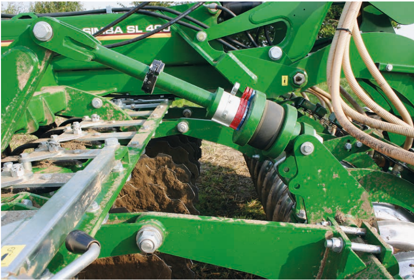
Figure 4: Depth adjustment by inserting spacers on two piston rods of the rear roller
