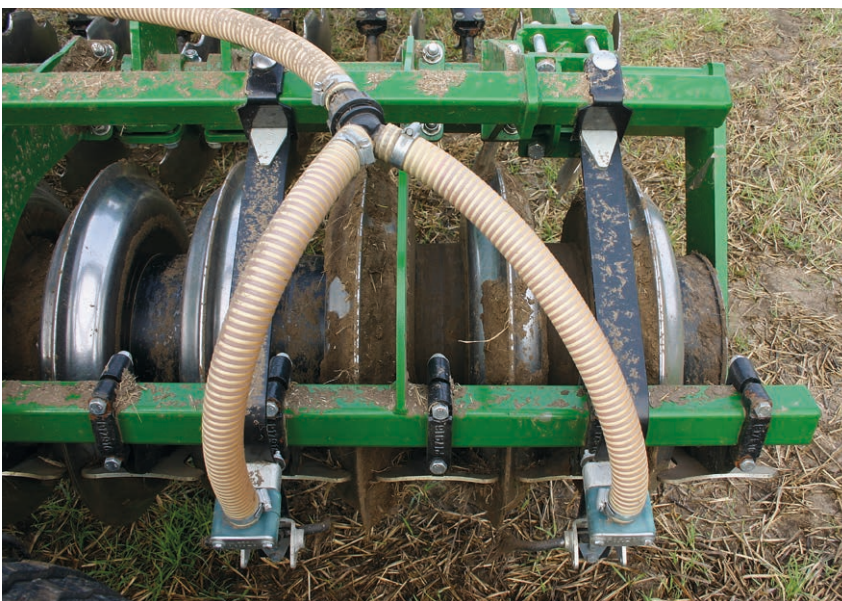
Figure 5: Rear roller – “Double Disc Light” steel packer roller with soil scrapers
