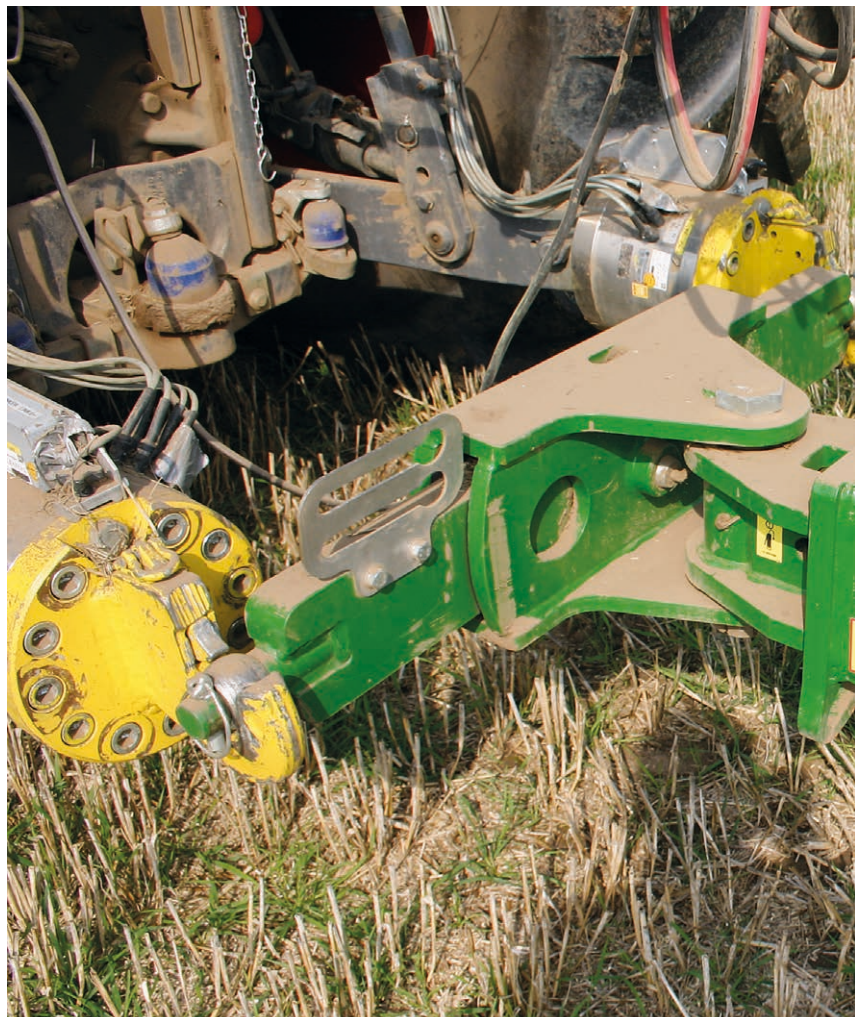
Figure 7: Facility for hanging hydraulic hoses when shutting down the short disc harrow
