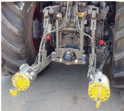
Figure 8: DLG 3D dynamometers for measuring the tractive force requirement
