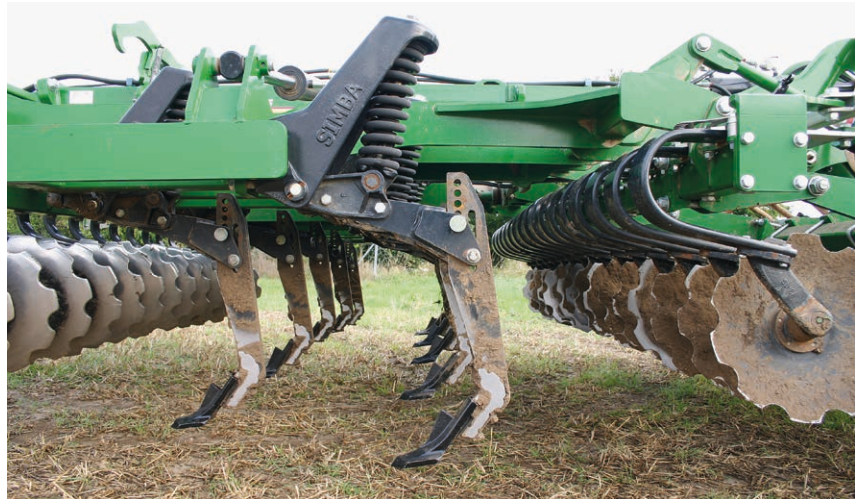
Figure 2: Front and rear rows of discs with conical concave discs, with cultivator tines fitted between them for deeper soil cultivation
