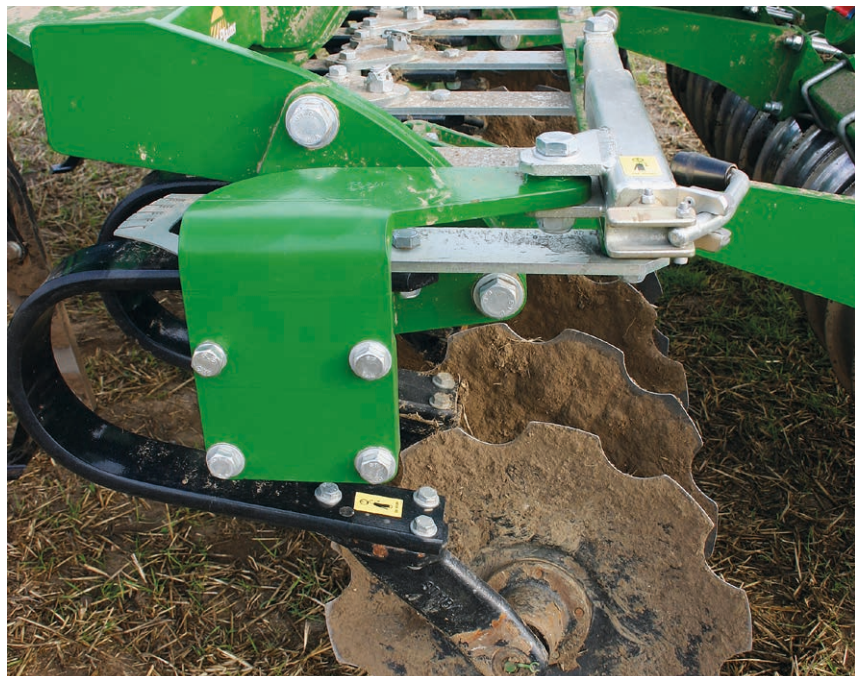
Figure 3: Disc cutting angle adjustment (shown here: rear row of discs)
