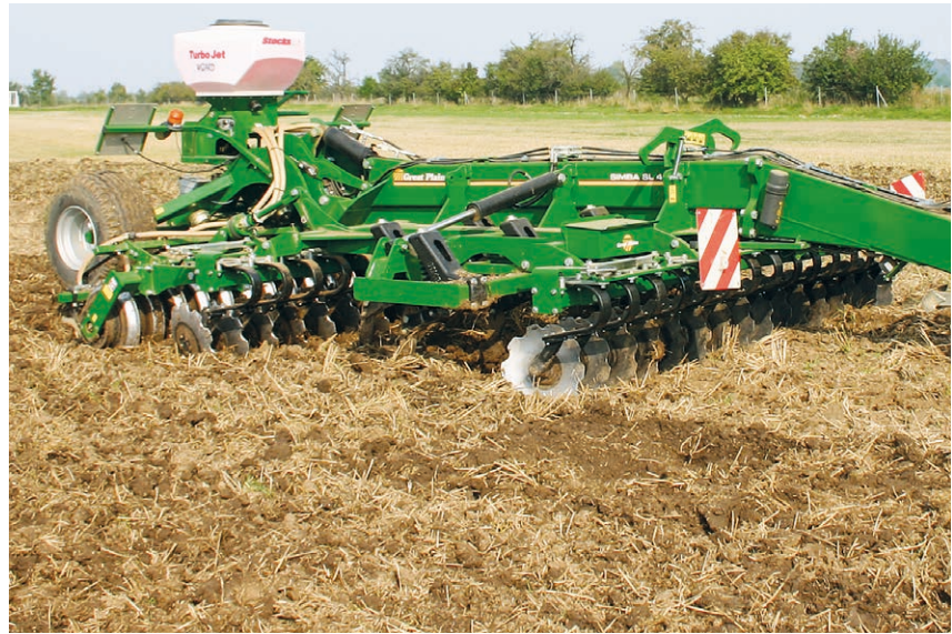
Figure 15: Cultivation pattern left behind by the SL 400 combination cultivator/disc harrow in the second working step (working speed: 9.3 km/h (3.7 mph))
