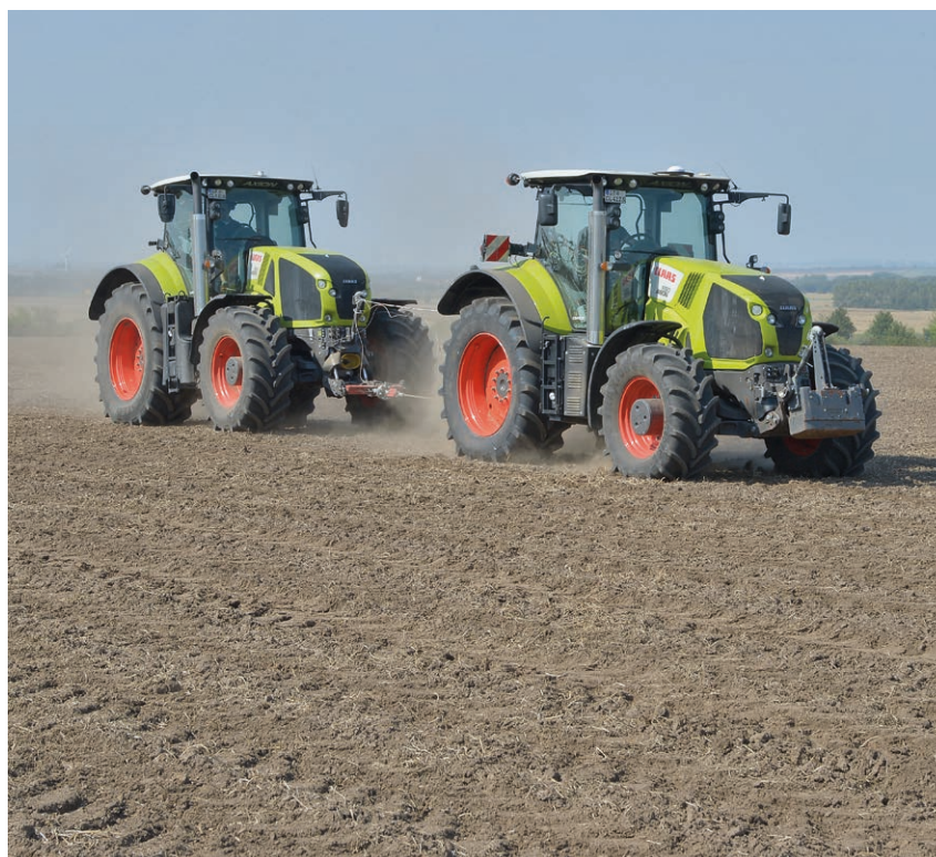
Figure 2: Towing tractor and braking tractor in the test to determine the traction and fuel efficiency in the field
