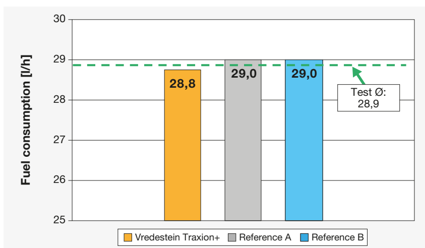
Figure 9: Results for absolute fuel consumption (DLG PowerMix transport cycles)
