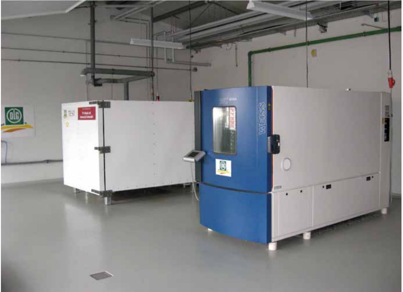
Picture 2: DLG test lab – two ammonia chambers
