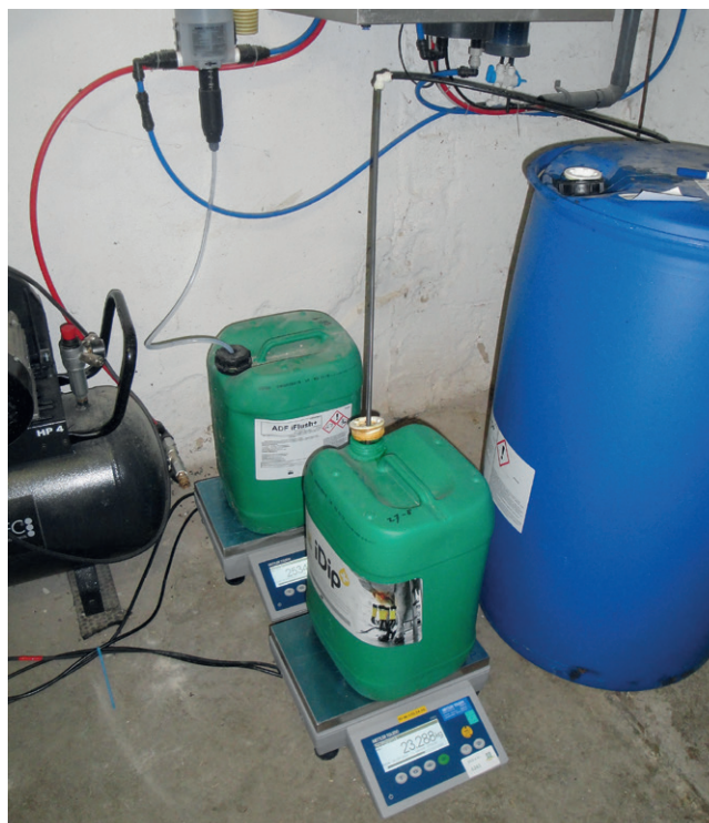
Figure 3: Measuring the difference in weight of the chemicals in use
