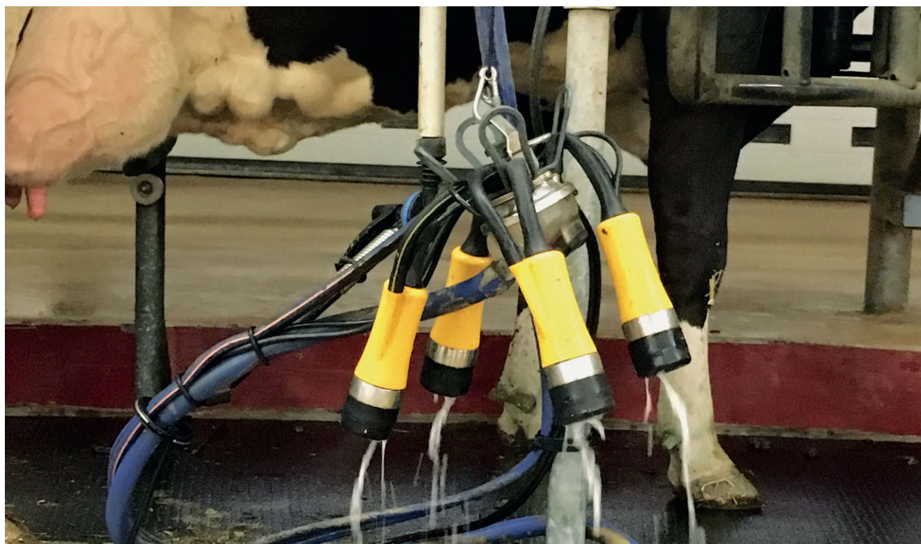
Figure 6: ADF 5 cluster during the flushing and disinfection
