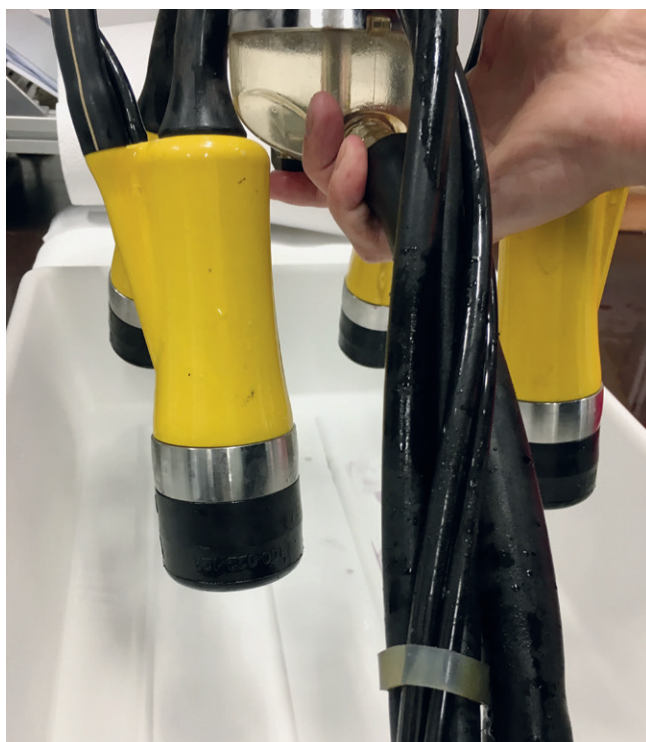
Figure 7: No coloured liquid residue after cleaning and disinfection between milkings
