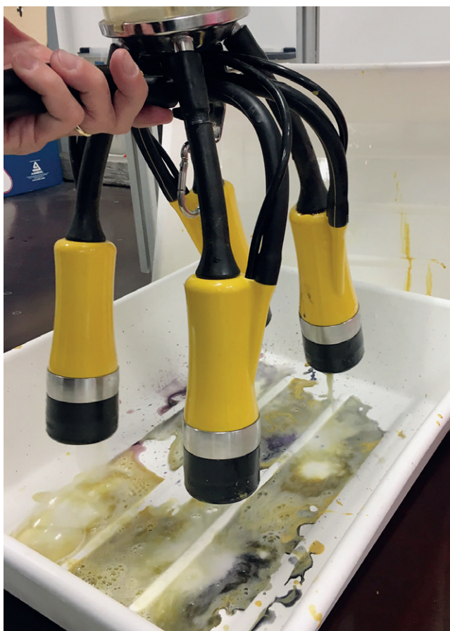
Figure 4: Iodine testing with starch solution
