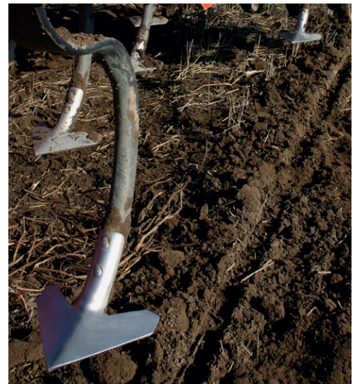
Figures 3 und 4: The tine points (left) and duckfoot shares (right) that were used in the DLG test
