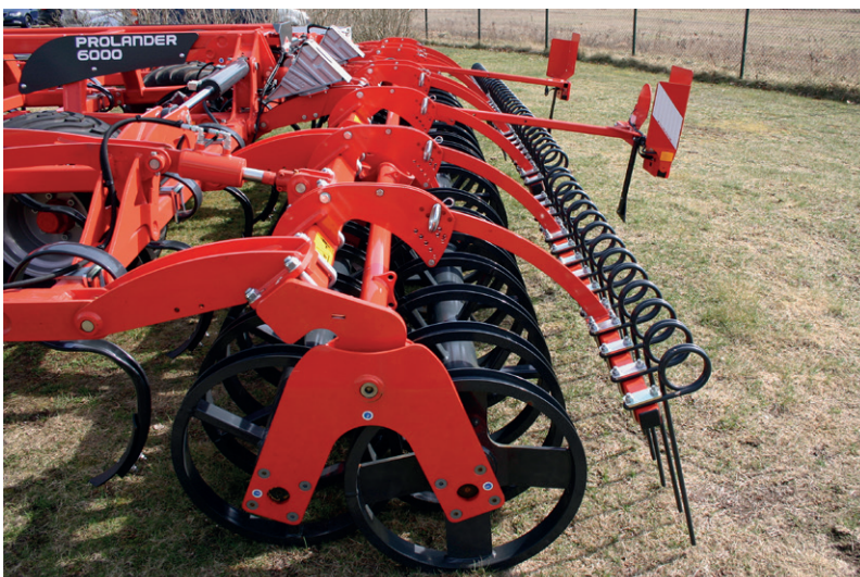
Figure 5: The trailing press with levelling tines
