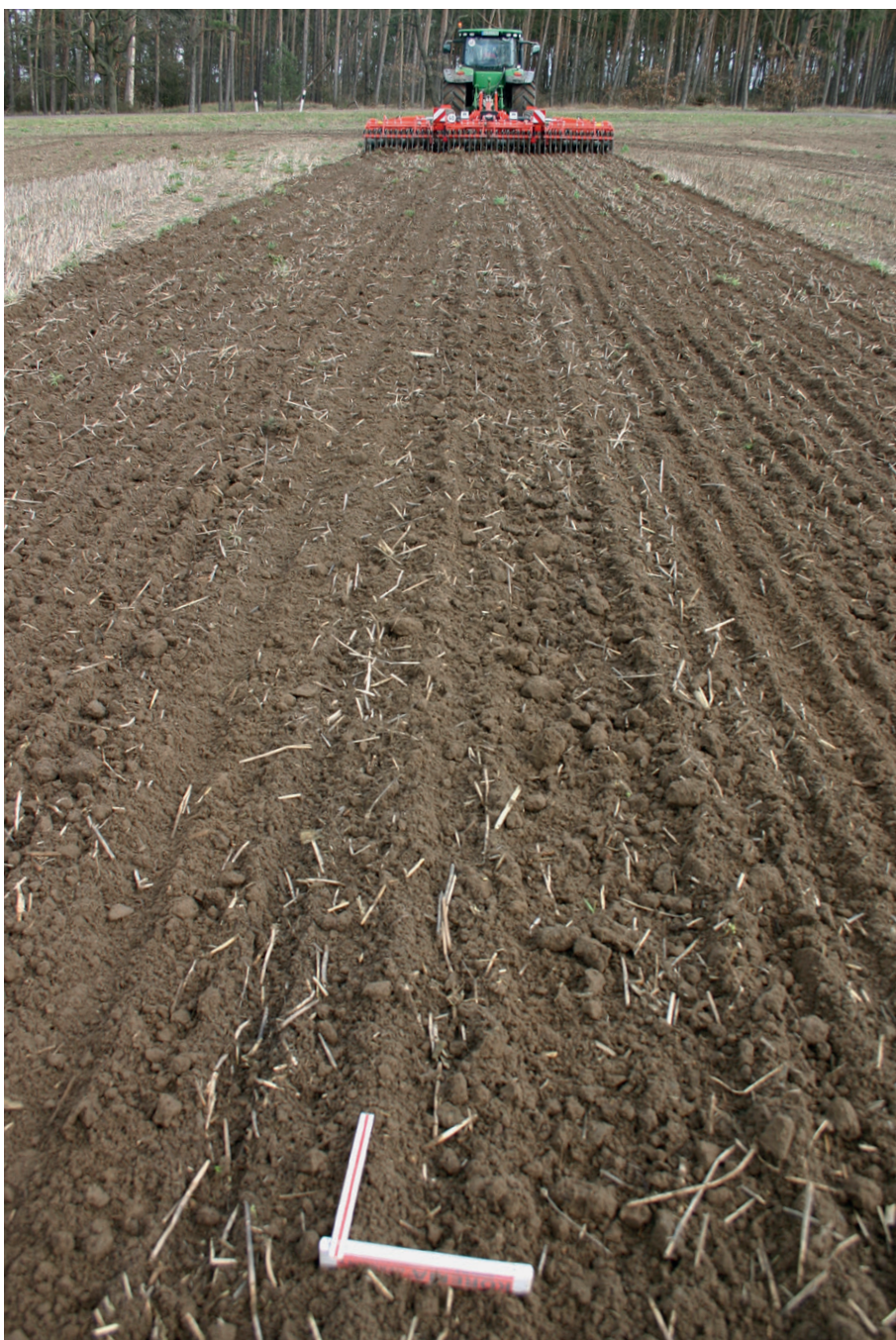
Figure 12: Quality of work in straw incorporation by the Kuhn Prolander (Forward speed: 9.5 km/h)
