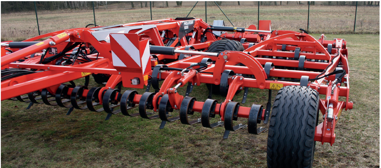
Figure 2: The leading bar with 22 levelling elements and hydraulic rams for height control
