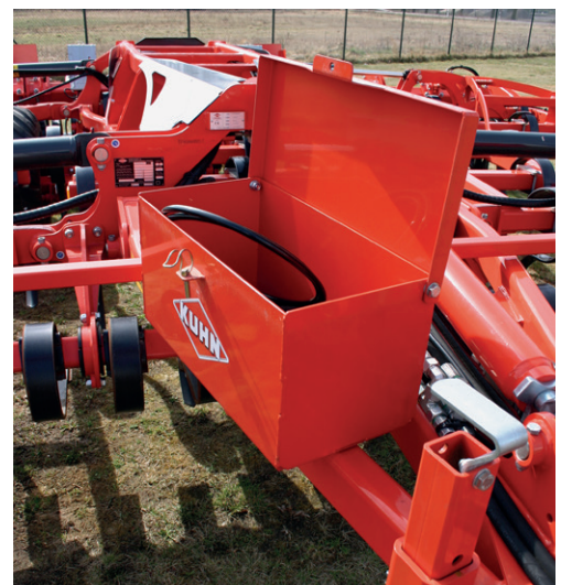
Figure 6: The box stores spare tines and tools
