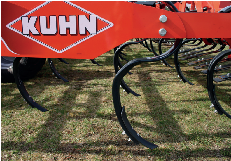
Figures 3 und 4: The tine points (left) and duckfoot shares (right) that were used in the DLG test
