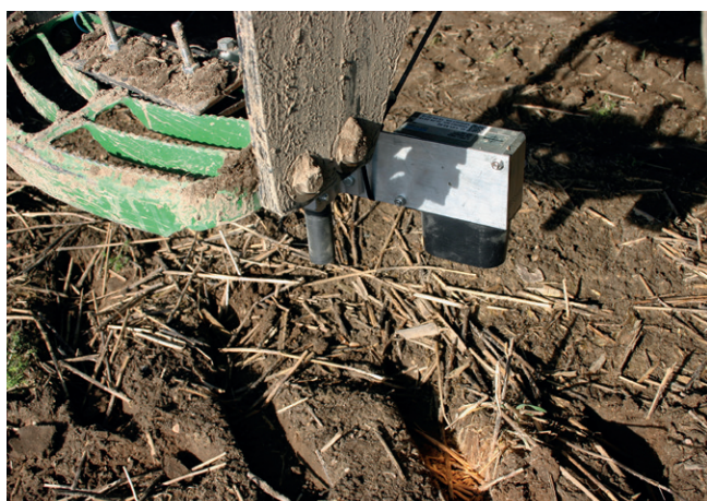
Figure 8: The Kistler Correvit L400 sensor
