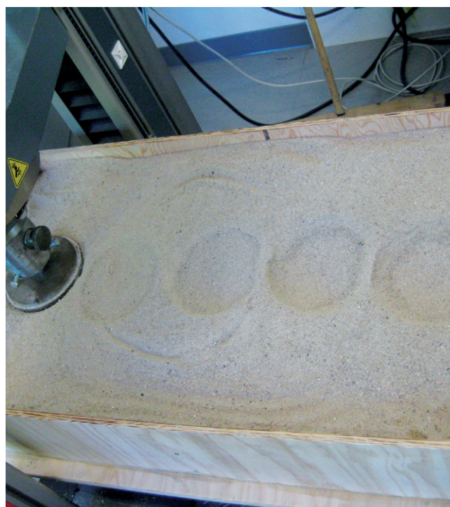
Figure 4: Measuring the deformability in new condition
