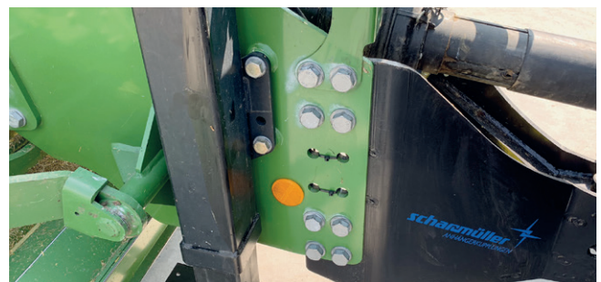
Figure 6: Hole pattern for installation
