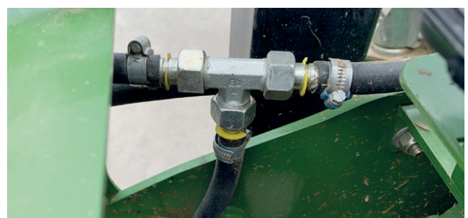
Figure 7: Compressed air connection adapter
