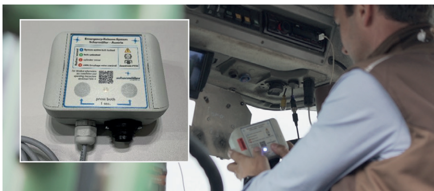
Figure 4: Cable remote control to be installed in the cab
