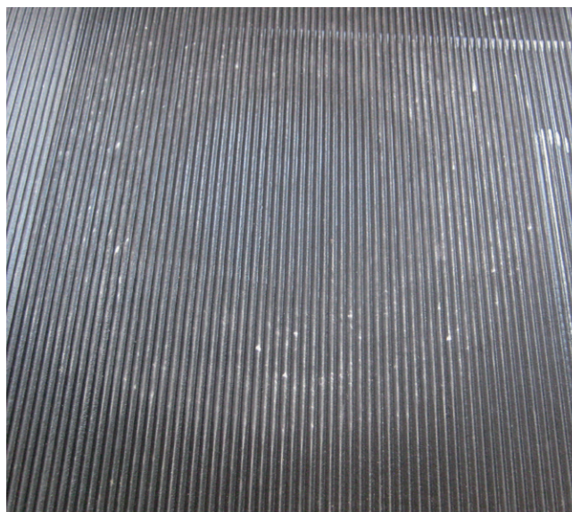
Figure 5: Underside of the mat – after permanent tread load test
