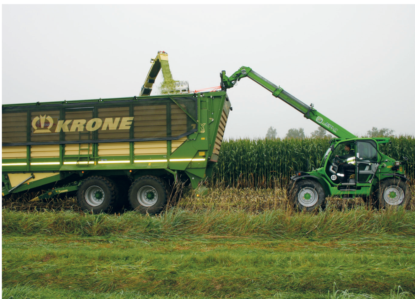
Photo 4: The chopped material is sampled as it exits the spout
