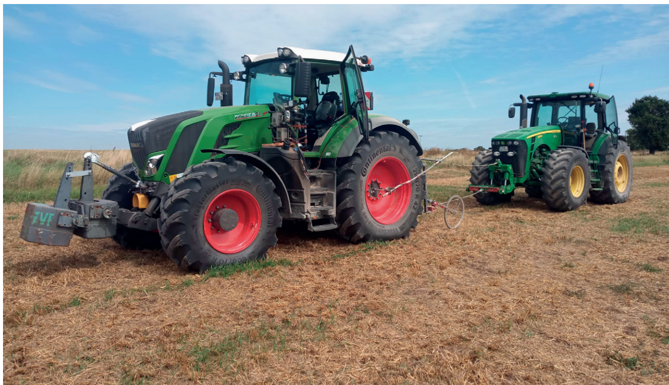
Photo 4: The test combination in field work – the Fendt 828 Vario is the test tractor that pulled the John Deere 8245R as the braked tractor
