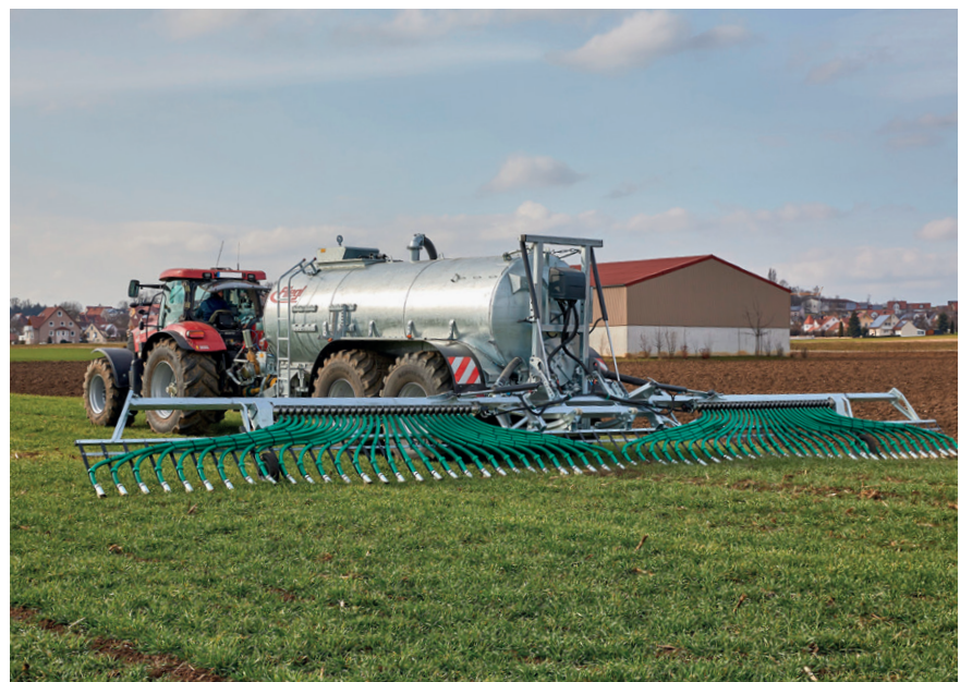
Figure 2: The trailing shoe applicator in work position
