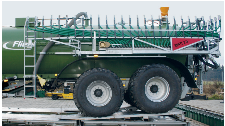
Figure 14: FLIEGL auger distributors on trailing shoe applicator FLIEGL SKATE 150 with hydraulically opening brass slide valve for emptying the traps
