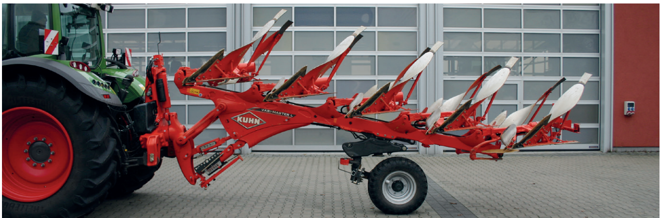
Fig. 5: The plough in transport position
