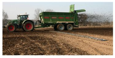
Fig. 2: The mobile test stand for measuring the distribution across rows
