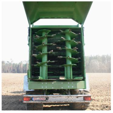
Fig. 6: 2-Spread has two vertical beaters with spreading discs on the bottom end
