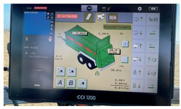
Fig. 4: The CCI 1200 terminal for BERGMANN M 6240 W with 2-Spread
