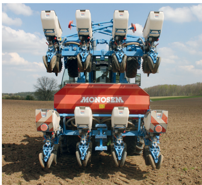
Fig. 3: The planter in transport position
