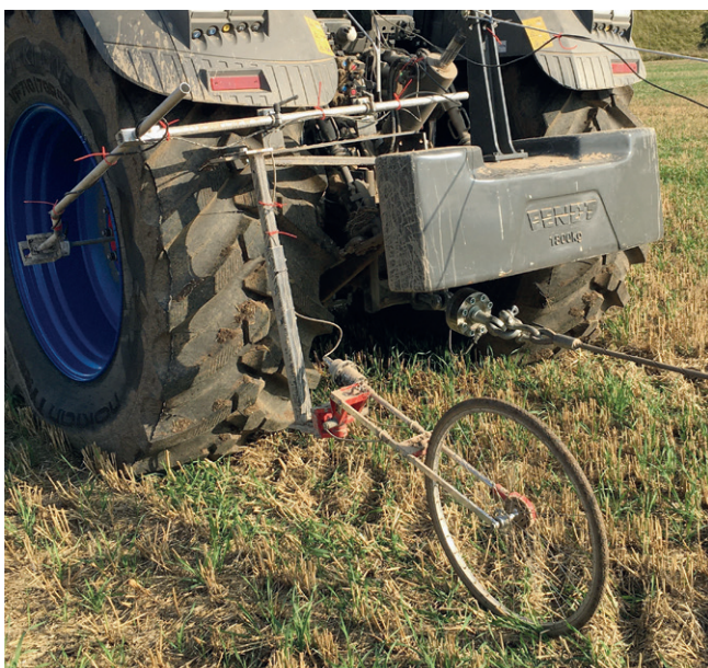
Figure 3: The measuring instruments on the test tractor – the sensor that measures the wheel rotations, the load cell and the Peiseler wheel (l.t.r.). The fuel consumption meter is not pictured
