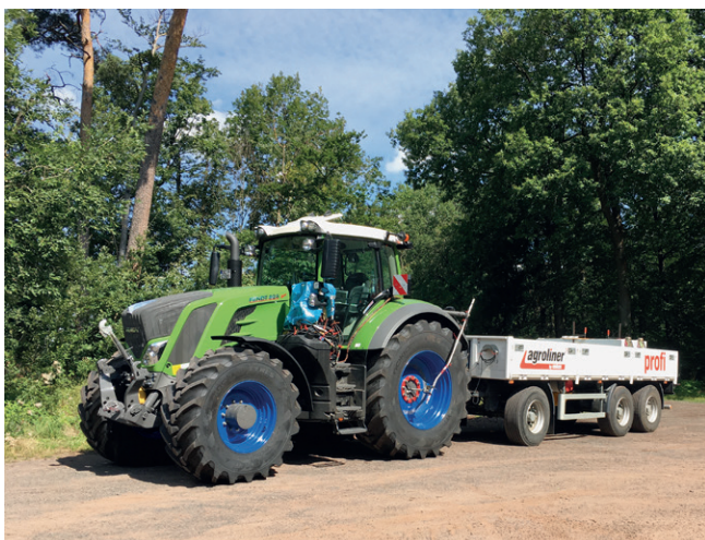
Figure 4: The test combination for the transport work tests
