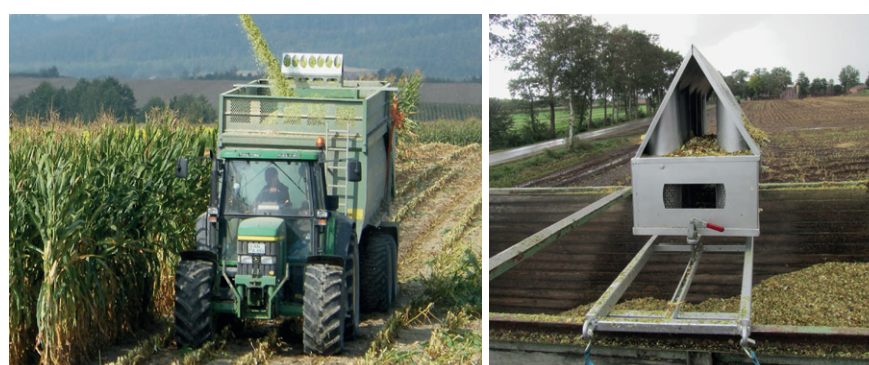
Figure 4: The DLG silage maize sampling unit is used for assessing the technical quality of chopping
