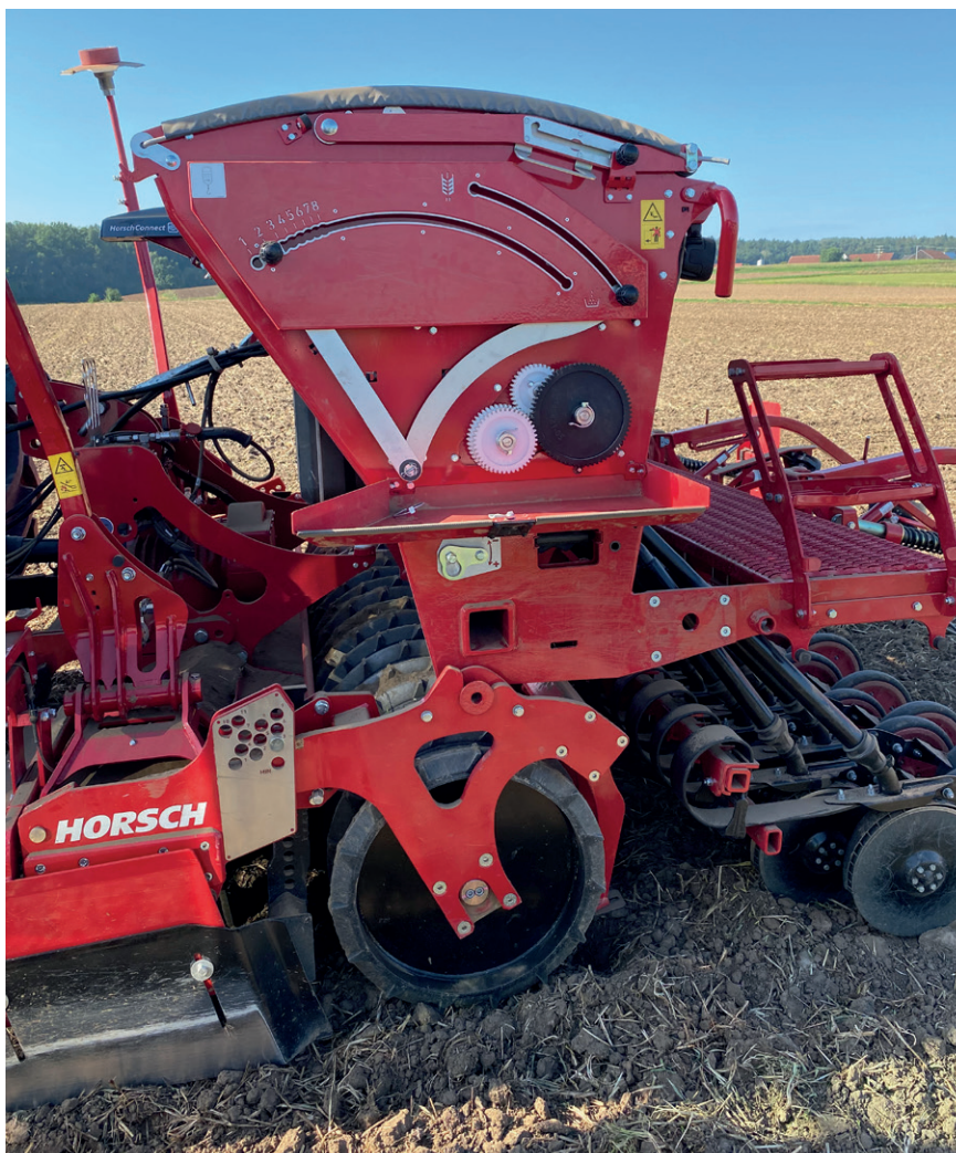
Figure 4: The Operating Centre on the Horsch Versa 3 KR drill
