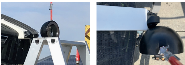
Figures 8 and 9: Impact test on the front-mounted camera
