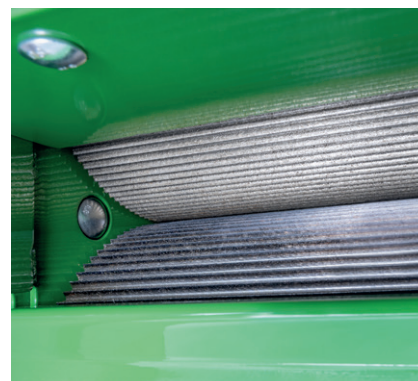
Figure 4: John Deere Premium High Intense 110/144 kernel processor
