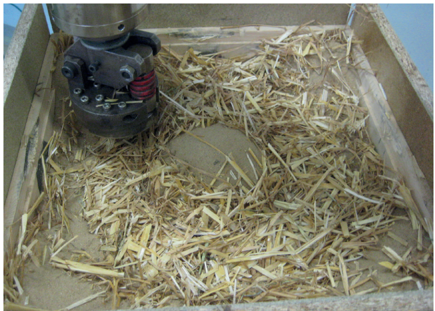
Figure 5: Permanent tread load test
