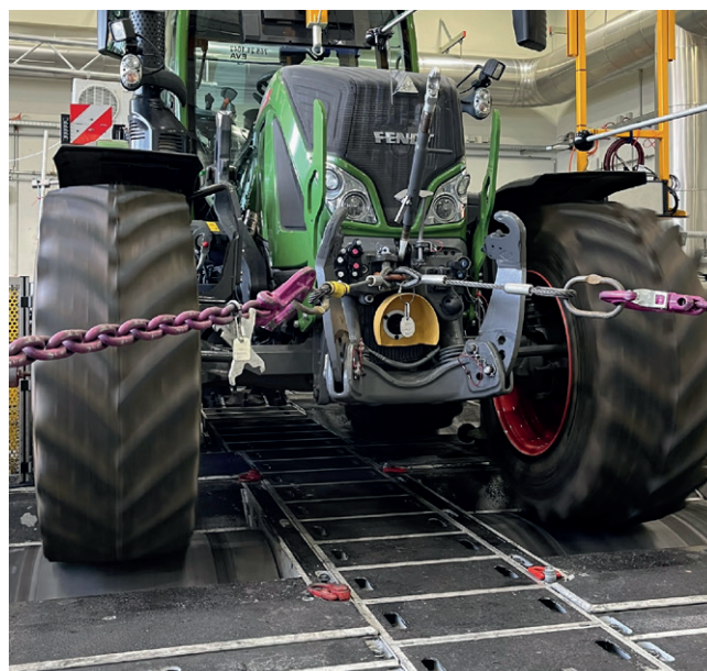
Figure 3: Tractor at the DLG rolling testbed
