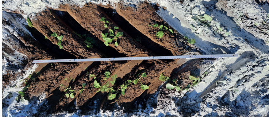
Figure 6: Dusted tire footprint area
