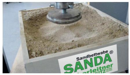
Figure 7: Measurement of deformability after permanent tread load
