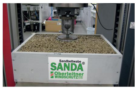
Figure 4: Measurement of deformability with straw pellet bedding in new condition
