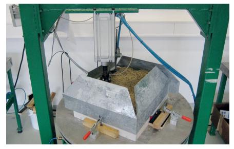
Figure 5: Permanent tread load test
