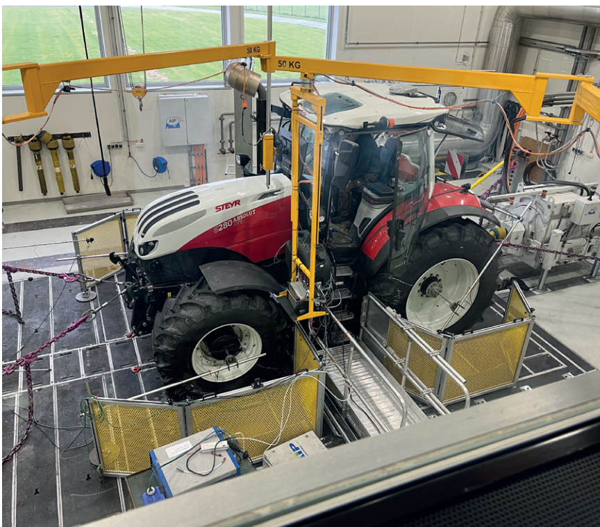
Figure 6: Transportation run on the DLG chassis dynamometer
