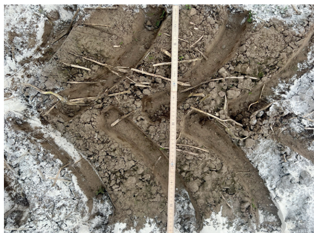
Figure 4: Wheel contact surface
