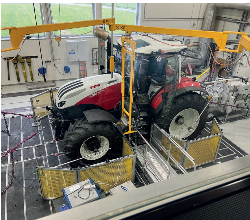
Figure 6: Transportation run on the DLG chassis dynamometer
