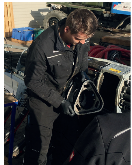
Fig. 16: The rotor with the macerator blades
