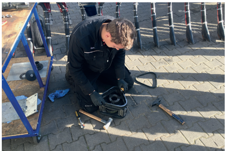
Fig. 18: Replacing the macerator blades
