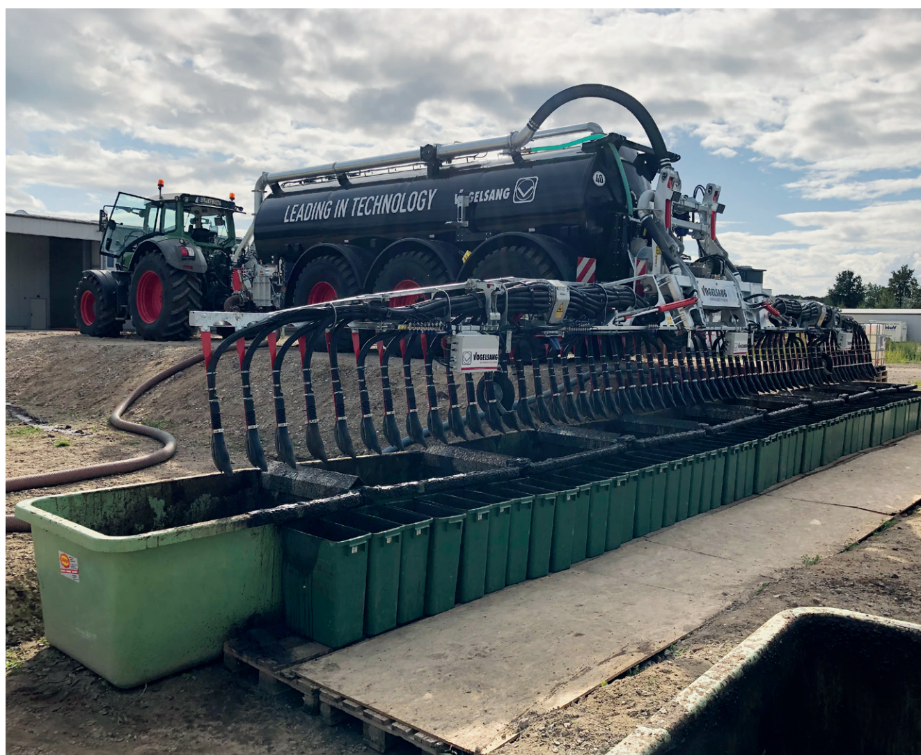
Fig. 4: The DLG test stand for measuring the distribution across rows (picture of the DLG test in 2019)
