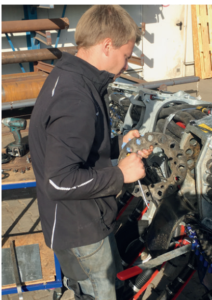
Fig. 17: Removing the macerator ring
