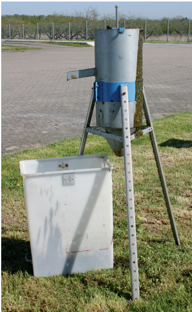
Fig. 5: The fluid meter for determining the ability to flow of the slurry
