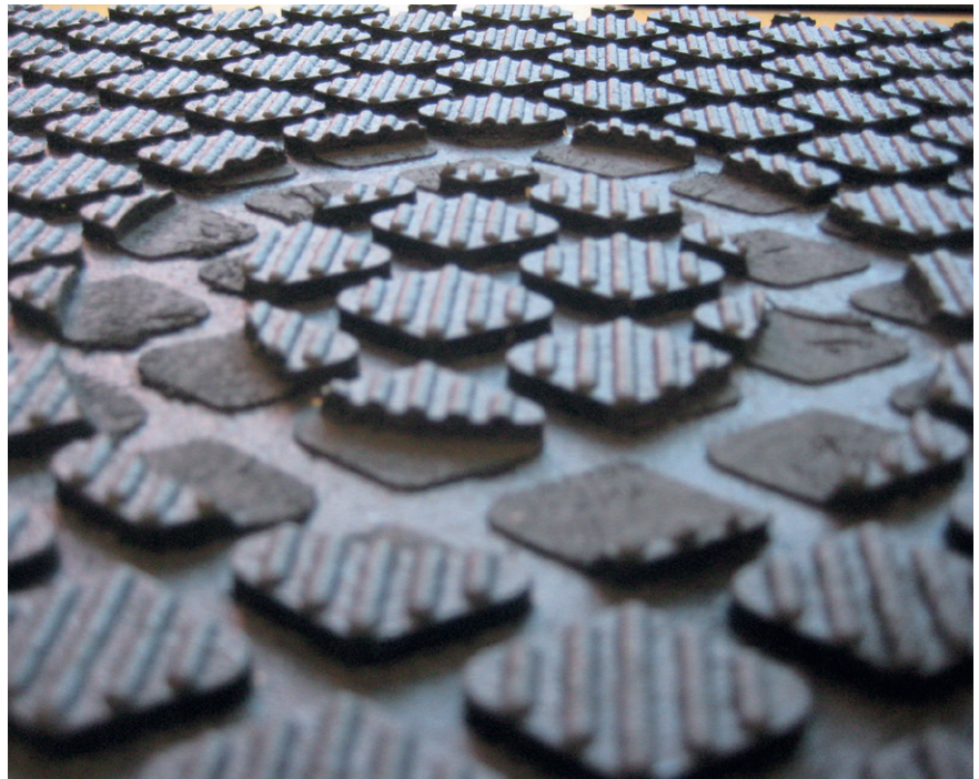
Figure 6: Test sample after abrasion test
