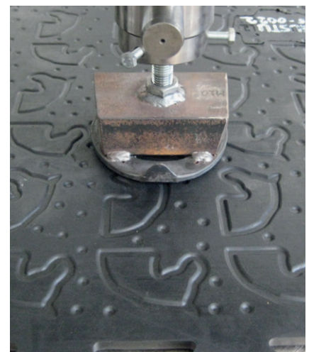
Figure 5: Deformation measurement with horseshoe
