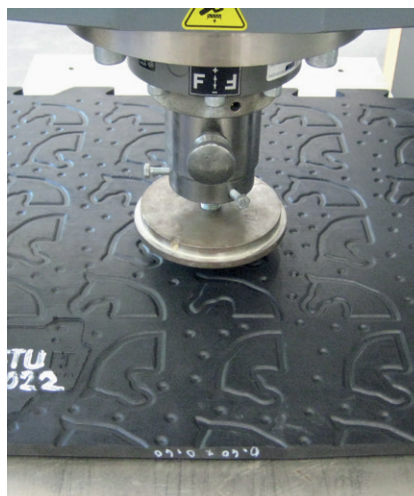
Figure 4: Deformation measurement with calotte
