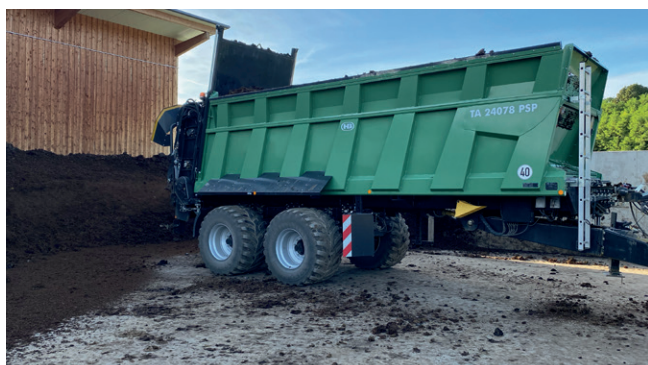
Figure 3: BRANTNER TA 24078 POWER-SPREAD pro during determination of longitudinal distribution
