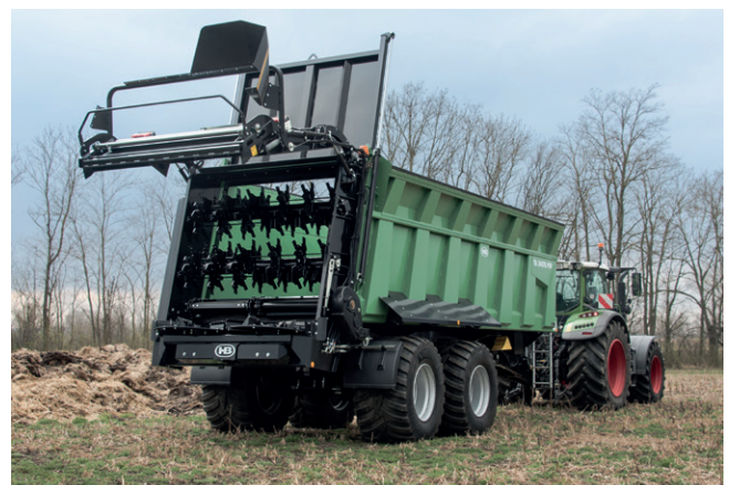
Figure 6: Universal spreading unit on the BRANTNER TA 24078 POWER-SPREAD pro
