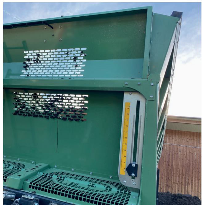
Figure 5: Display on the front panel of the spreader for the opening height of the damper valve
