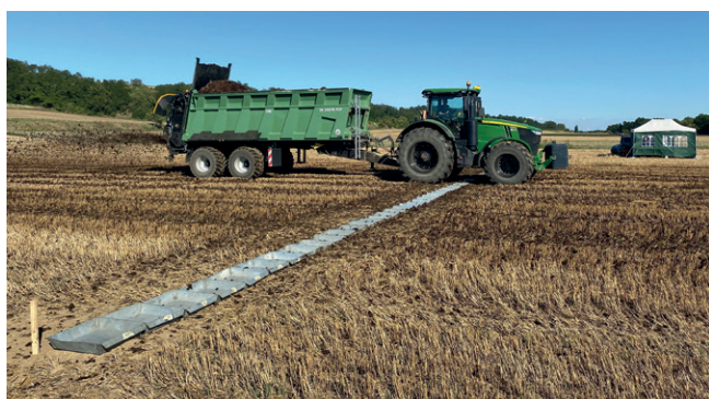
Figure 2: Mobile test bench for determining transverse distribution
