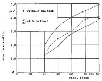
Speed before application of brakes, without ballast  $$40,3\ km/h$$  with ballast  $$39,9\ km/h$$
