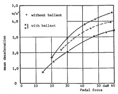
Speed before application of brakes, without ballast 24,7 km/h with ballast 24,7 km/h
