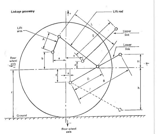
Dimensions of Linkage Geometry (When Connected to the Standard Frame) mm
