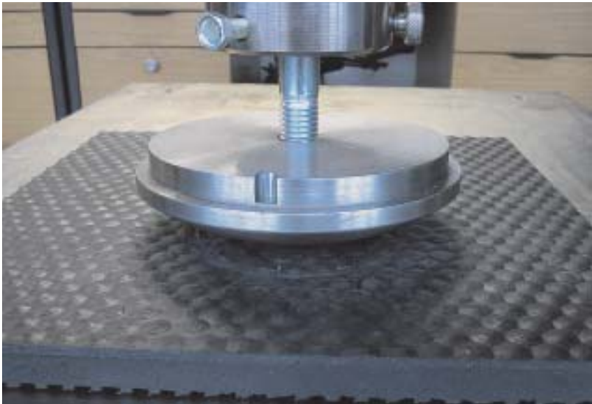
Figure 3: Measurement of deformability with a calotte
